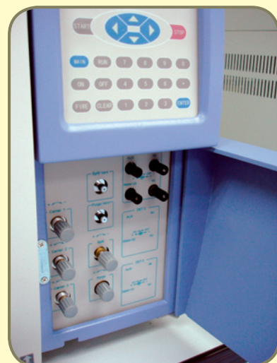
Carrier gas and detector gas flow control
